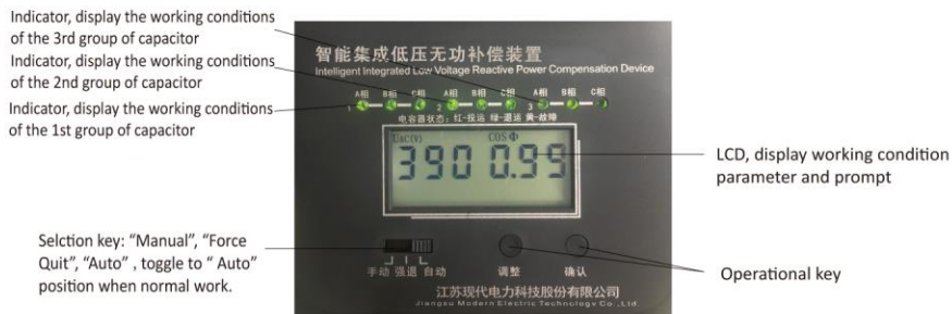
Figure 7-2 Panel layout of D-type product
