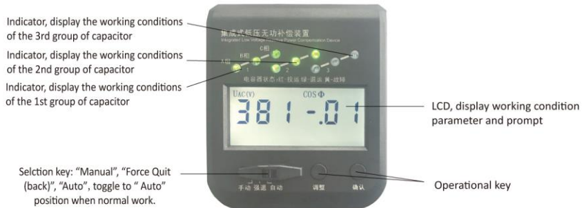
Figure 7-1 Panel layout of X-type product
